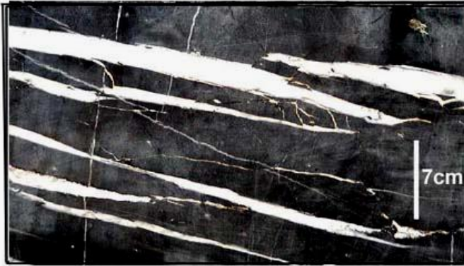
(1) This type of black limestone exist in both Qulqula Radilarian Formation and in Jurassic units ( e.g. Sargelu Fn ). But the closest to the marble quarries is the former one. The white areas are calcite filled tension gash fractures arranged nearly in an echelon pattern. It's metamorphism yield the similar below marbles.
