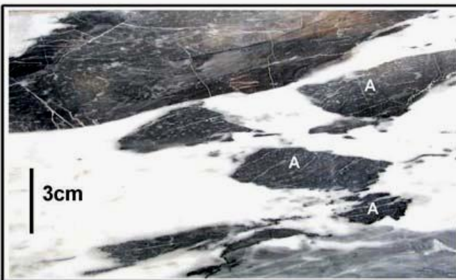
(2) Black marble with white spots shows slight degree of homogenization and deformation. The areas indicated by ( A ) are fragments of background in the white calcite.
