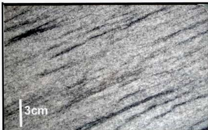
(4) Gray marble originated from diagenetic and metamorphism processes. The first includes solution of limestone under burial pressure or tectonic stresses and development of non-sutured solution seams ( black discontinuous lines). while the second one includes recrystallization and some degrees of homogenization with compaction. These type of marbles exist in Rawkan, Gmo and Darashimana area.
