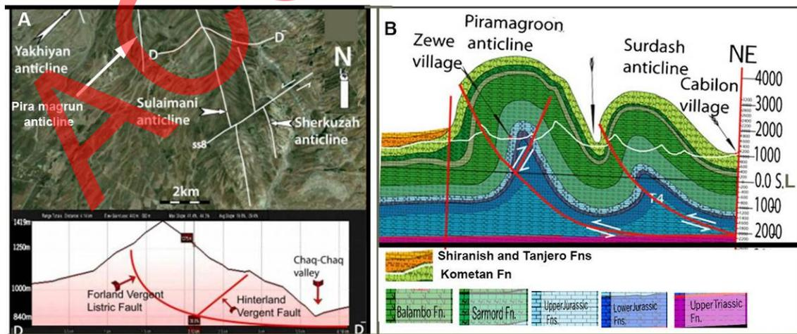
Figure(13)Two geological cross sections of A)Al-Hakari (2011) and B)Al-Hakari (2011); Omer *et al.*(2015)shows that they assigned the anticlines in studied area as fault propagation folds which uplifted through the reverse slipping of the hanging wall of the blind foreland vergent listric thrust fault associated with the hinterland-vergent-fault.
