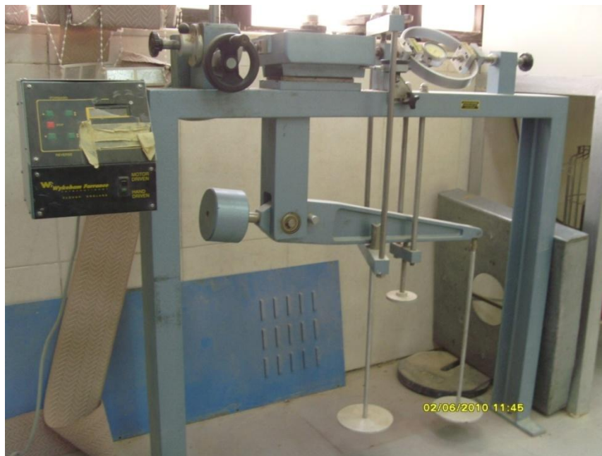
Figure (3-1) Shear box test apparatus
