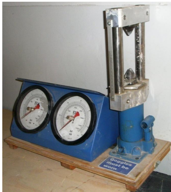
Figure (3-3) Point load test apparatus (ELE)model
