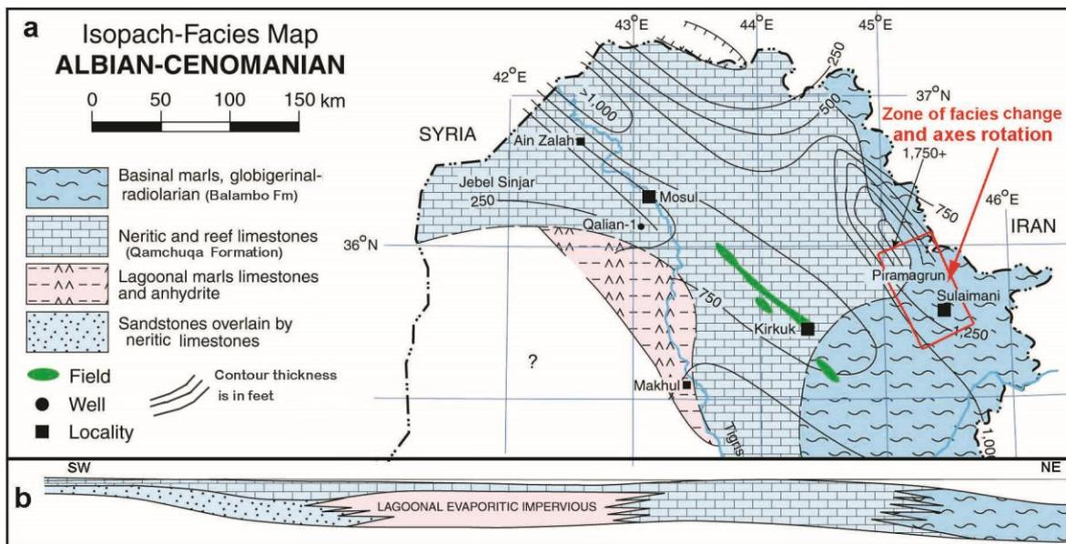
Fig. (4) A map of the Cretaceous facies change (Dunnington, 1958) [17] on which the studied area and rotation of anticline axes are indicated
